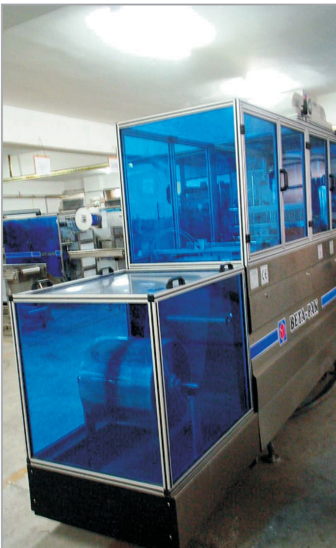
Filling and Packaging Machine Cabinet
