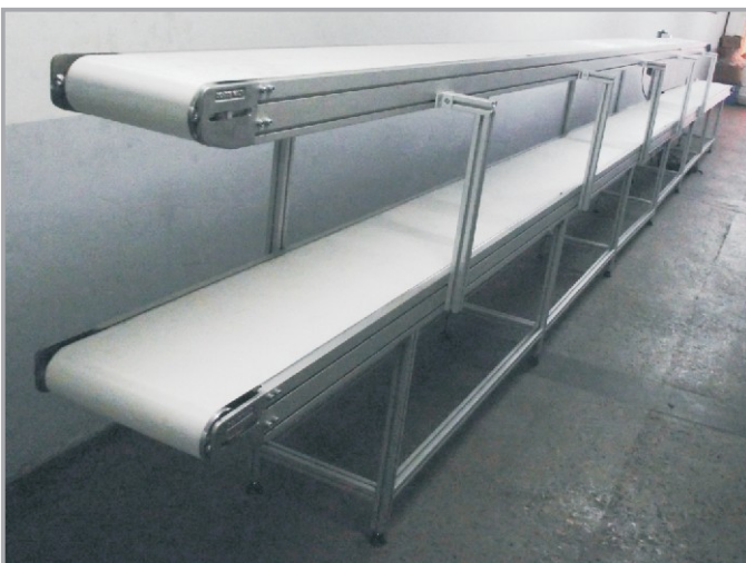
Double Deck Conveyor
